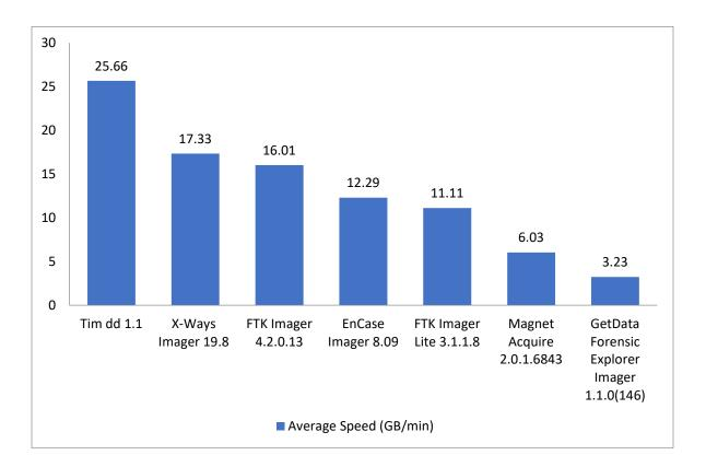
SummaryAll verified forensic images created have shown consistent imaging speeds relative to the tool being used to assure repeatable and reliable results. Imaging with our write-blocked USB 3.1 HotSwap trays in conjunction with devices on the UltraBay greatly increases the forensic imaging capacity of each FRED system, which in turn frees up more imaging equipment in your lab and provides you with more
